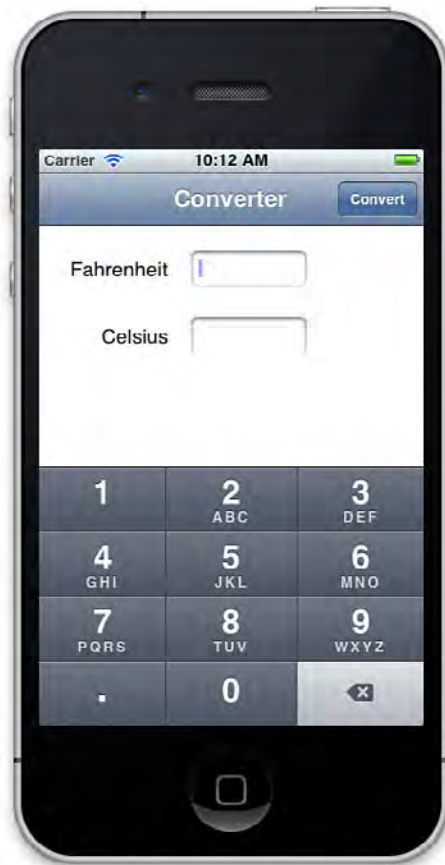
Figure 4-13 By assigning UIKeyboardTypeDecimalPad to a field's keyboard type, you allow this keypad-style keyboard to limit a user's entry to numbers and a decimal point.
