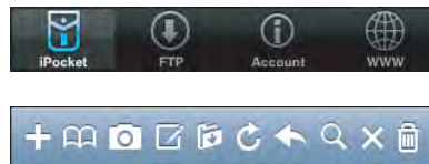
Figure 4-3 Tab bars are 48 points high for 320×480-point iPhone and iPod units (top). Toolbars use the same 44-point spacing as standard navigation bars.
