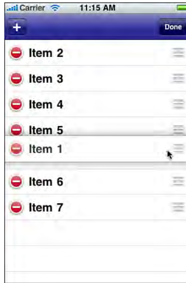
Figure 11-8 Reorder controls appear at the right of each cell during edit mode. They appear as three stacked gray lines. This screenshot shows Item 1 being dragged into place below Item 5.
