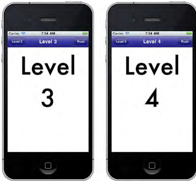
Figure 5-3 The navigation controller automatically creates properly labeled back buttons. After the Level 4 button is selected in the left interface, the navigation controller pushes the Level 4 view controller and creates the Level 3 back button in the right interface.
