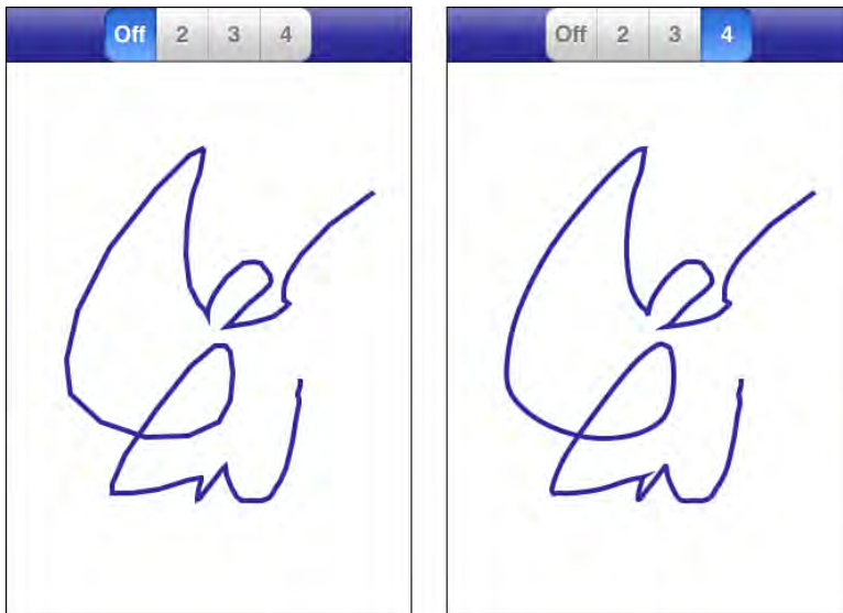
Figure 8-5 Catmull-Rom smoothing can be applied in real time to improve arcs between touch events. The images shown here are based on an identical gesture input, with and without smoothing applied.
