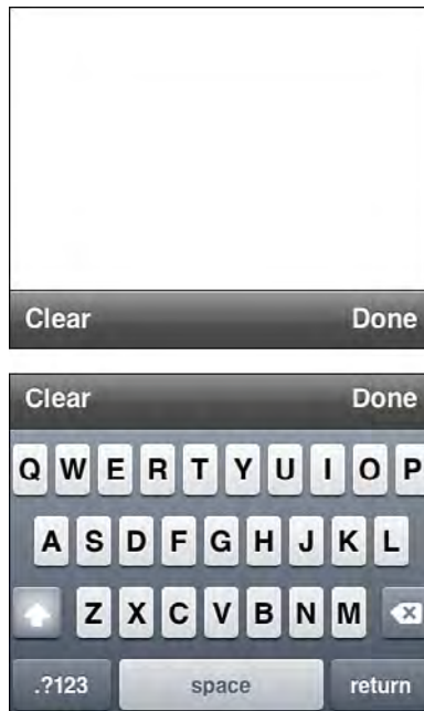
Figure 10-5 When a hardware keyboard is detected, the keyboard is dismissed but not the accessory view, which remains onscreen at all times that its owner view holds first responder.
