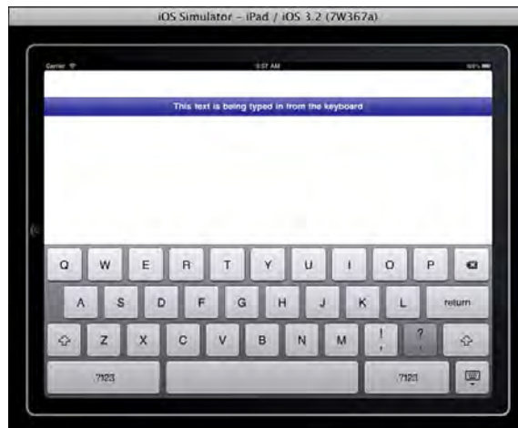
Figure 10-8 Adding the UIKeyInput protocol to a toolbar transforms the view into one that can accept and display keyboard input, including deletions.
