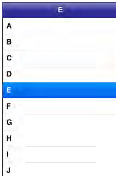
Figure 11-1 It's easy to fill a UITableView with cells based on any array of strings. This table contains letters, which it presents as a flat list without sections.
