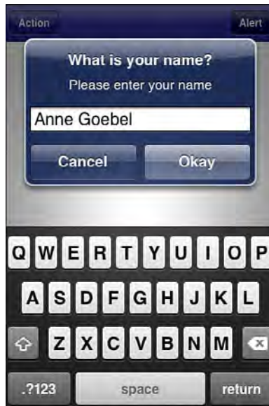
Figure 13-3 This modal alert returns immediate answers because it's built using its own run loop.
