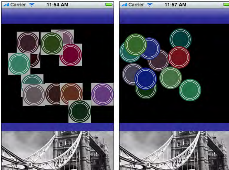
Figure 8-2 The application should ignore touches to the gray areas that surround each circle (left). The actual interface (right) uses zero alpha values to hide the parts of the view that are not used.
