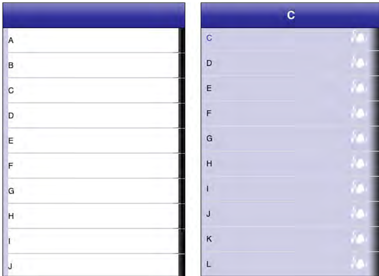
Figure 11-3 Table cell labels will obscure background art unless the table's background color is set to clear.
