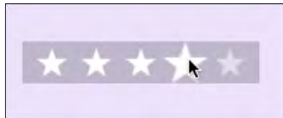
Figure 9-9 Recipe 9-6 creates a custom star slider control that animates each star upon selection. A simple animation block causes the star to zoom out and back as the control’s value updates.
