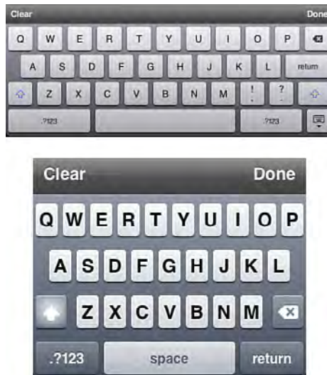
Figure 10-4 Accessory input views allow you to add custom view elements to standard iOS keyboard presentations. Here, a pair of buttons augment iPad and iPhone keyboards.
