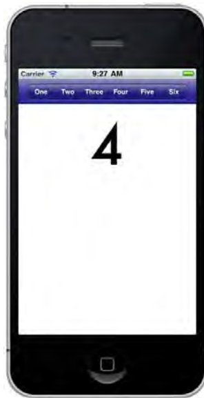
Figure 5-2 Adding a segmented control to the custom title view allows you to build a multi-item menu. Notice that no items remain highlighted even after an action takes place. (In this case, the Four button was pressed.)
