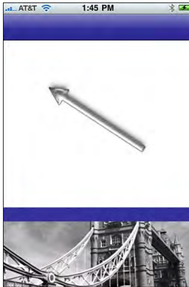
Figure 14-1 A little math recovers the “up” direction by performing an arctan function using the x and y force vectors. In this example, the arrow always points up, no matter how the user reorients the iPhone.
