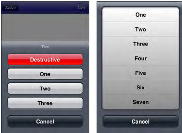
Figure 13-4 On the iPhone and iPod touch, action sheet menus slide in from the bottom of the view. Although the Destructive menu button appears gray here (left), it is red on iOS devices and indicates permanent actions with possible negative consequences to your users. Adding many menu items produces the scrolling list on the right.
