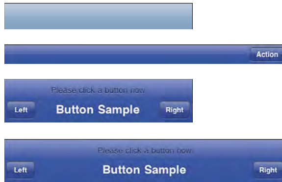
Figure 4-2 Navigation bars stretch from one side of the screen to the other. Their height is fixed at 44 points (32 points for landscape on iPhone and iPod touch). The rarely used prompt feature (shown in the bottom two images) zooms the bar to 74 points high.
