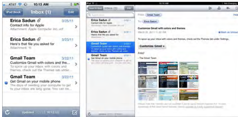
Figure 5-1 The iPhone's Navigation Controller uses chevrons to indicate that detail views will be pushed onscreen when their parents are selected.
