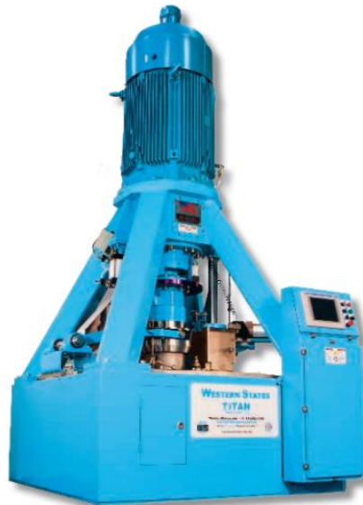
Fig. 4. Centrifuga TITAN discontinua.(Western States Machine Company, 2020)
