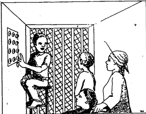
High position of control panel
