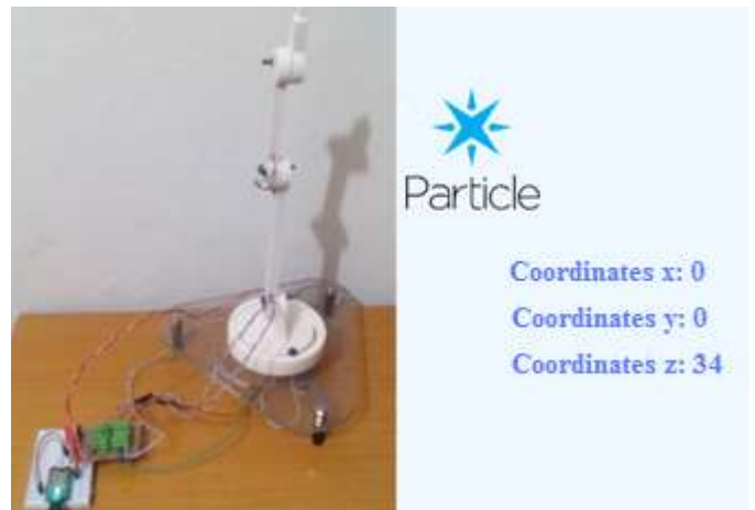
Fig. 11. Verification of Cartesian coordinates in haptic device via web interface.
